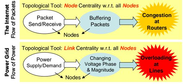
Fig. 3. Contrast between packet congestion in Internet and line overloading in power grid.
