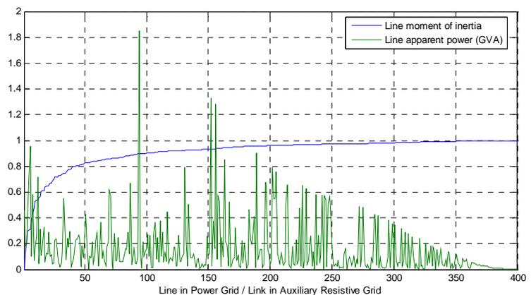
Fig. 5. Apparent power flow vs. moment of inertia for different lines in the power grid.
