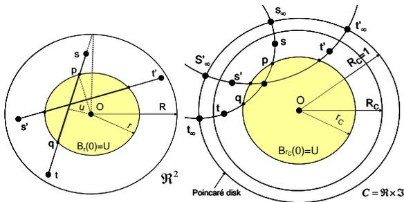
Fig. 1. ‘Traffic’ on Euclidean (left) vs. Poincaré (right) space. The optimal paths are uniformly distributed in a Euclidean space, but maximally distributed at the center in a Poincaré space.
