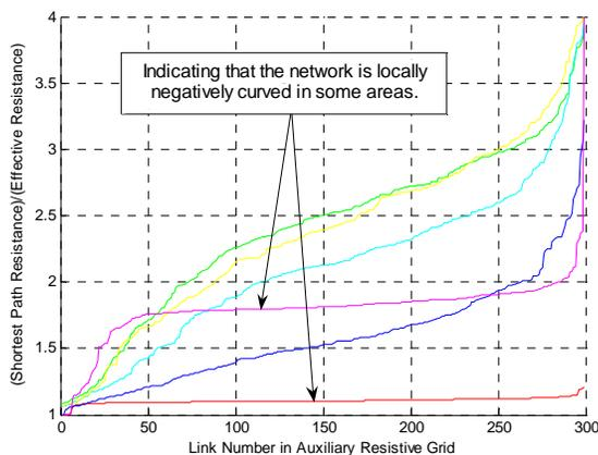
Fig. 4.  $R(x_k, x_i)/R_{eff}(x_k, x_i)$  for five nodes in auxiliary resistive grid.
